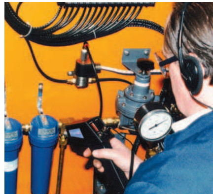
2 Detect air leak-ages with SKF Ultrasonic Leak Detector CMIN 400
