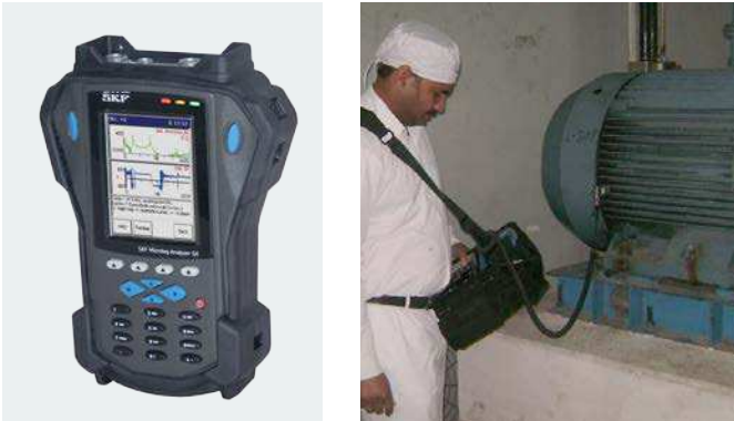
Periodic data collection with SKF Microlog Analyzer
