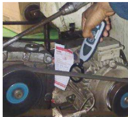
4 Detect electrical discharge with SKF Electrical Discharge Detector pen TKED 1
