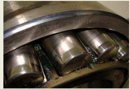
After 10 years of operation in a sugar mill exhaust fan, this CARB toroidal roller bearing continues to provide superior performance.
